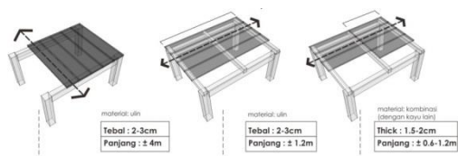
Figure 7. Development of walkways material
